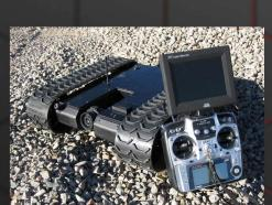
Optional accessories include a 4 axis manipulator arm, thermal camera, PTZ camera, drive camera, rear-facing camera, 2-way audio, remote detachable trailer, lights, and an assortment of gripper tools. (hook, box knife, doorknob-fingers and spreader) The robot is capable of operating in harsh conditions, and can be customized to perform a wide range of tasks.
